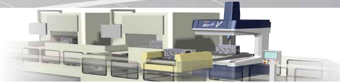
Mach and Mach-V CMMs are designed for in-line manufacturing processes
