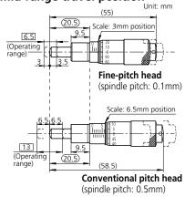
While the fine-pitch micrometer head has a measuring range of 6.5mm, the conventional head has a larger range of 13mm. When replacing a conventional head, the fine-pitch type can use the common range in the middle of the spindle travel. The standard and compact types of fine-pitch head are completely interchangeable.
