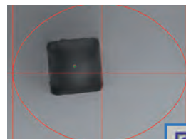
Area Centroid Tool This tool evaluates the position of a feature's centroid. It is appropriate for capturing the center of a feature.
