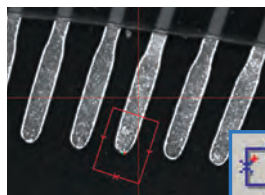
Maximum/Minimum Tool This tool evaluates the maximum or minimum point within the range.
