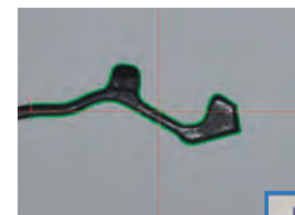
Auto Trace Tool This is a form measuring tool that can autonomously track an unknown feature.
