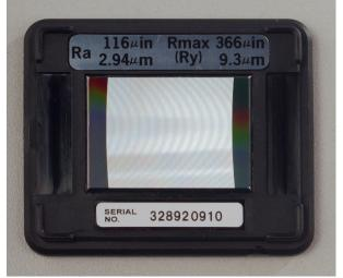
Problem: Comparators are limited to a single Ra parameter. When parameters or machine processes change, comparators become obsolete. Part drawings can specify a number of different parameters depending on the application of the part. Profilometers can calculate roughness values according to the print such as: the arithmetic average (Ra), root mean squared (Rq), highest peak (Rp), deepest valley (Rv), max peak to valley (Ry), etc.
