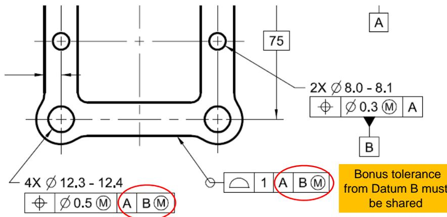
Patterns, simultaneous requirement, and M on datums can create measurement challenges.
