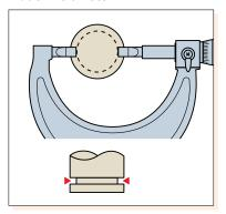
For diameter inside narrow groove measurement
