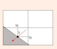
Detected edge position (from the center of vision) V = (Vx, Vy)
