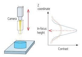
The AF system analyzes an image while moving the Camera up and down in the Z axis. In the analysis of image contrast, an image in sharp focus will show a peak contrast and one out of focus will show a low contrast. Therefore, the height at which the image contrast peaks is the just-in-focus height.
