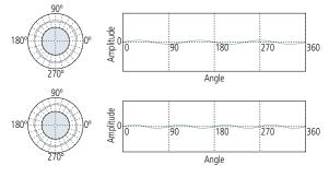
A 5 to 15 UPR condition often indicates unbalance factors in the machining method or processes used to produce the workpiece.
