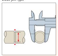
For diameter of narrow groove measurement
