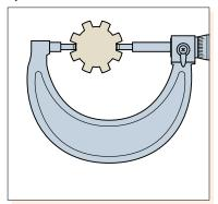
For splined shaft diameter measurement
