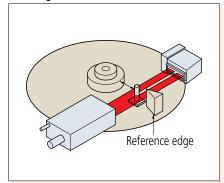
Measurement of outer diameter of optical connector and ferrule
