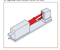
Measurement of outer diameter and roundness of cylinder
