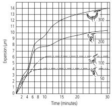
The above graph shows micrometer frame expansion due to heat transfer from hand to frame when the frame is held in the bare hand which, as can be seen, may result in a significant measurement error due to temperature-induced expansion. If the micrometer must be held by hand during measurement then try to minimize contact time. A heat insulator will reduce this effect considerably if fitted, or gloves may be worn. (Note that the above graph shows typical effects, and is not guaranteed).
