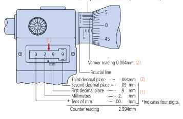
Note) 0.004 mm (2) is read at the position where a vernier graduation line corresponds with one of the thimble graduation lines.
