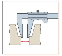
For outside diameter measurement such as thickness of recess
