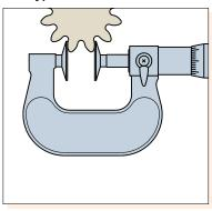
For root tangent measurement on spur gears and helical gears.
