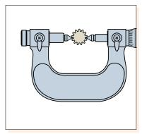
Measurement of gear over-pin diameter
