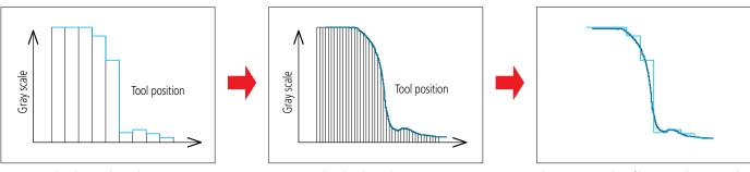
Image signal without sub-pixel processing
