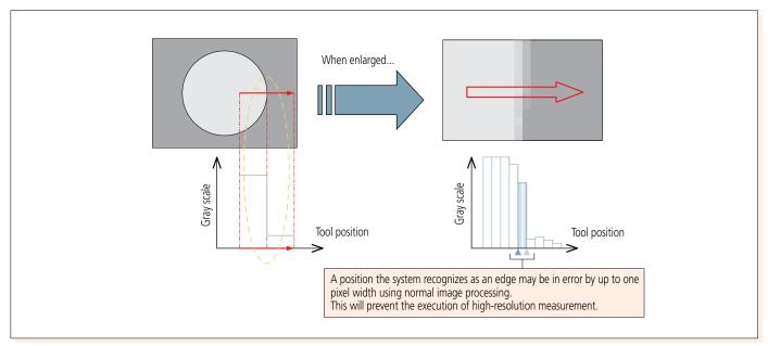
To increase the accuracy in edge detection, sub-pixel image processing is used. An edge is detected by determining interpolation curve from adjacent pixel data as shown below. As a result, it allows measurement with a resolution higher than 1 pixel.
