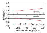
Figure 3 Repeating range of length measurement
