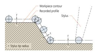
If a profile is read from the recorder through a template or scale, it is necessary to compensate for the stylus tip radius beforehand according to the applied measurement magnification.
