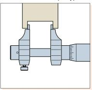
For small internal diameter, and groove width measurement
