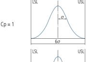
The process capability is barely achieved as the 6 sigma process limits are coincident with the tolerance limits.
