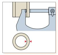
For pipe thickness measurement
