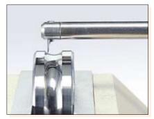
Inner/outer ring contour of a bearing
