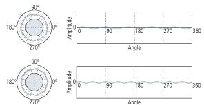
A 15 (or more) UPR condition is usually caused by tool chatter, machine vibration, coolant delivery effects, material non-homogeneity, etc., and is generally more important to the function than to the fit of a workpiece.
