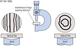
Measuring face is curved by approximately  $1.3\mu m$ . (0.32 $\mu m$  x 4 paired red fringes.)
