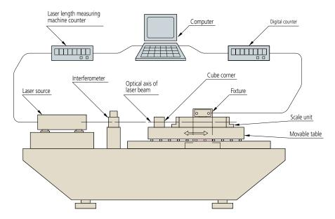
The accuracy of the scale at each point is defined in terms of an error value that is calculated using the following formula:
