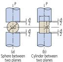
Assuming that the material is steel and units are as follows: Modulus of elasticity: E=205 GPa Amount of deformation:  $\mathcal{O}(\mu m)$  Diameter of sphere or cylinder: D (mm) Length of cylinder: L (mm) Measuring force: P (N) a) Apparent reduction in diameter of sphere  $\mathcal{O}_1=0.82\ \tilde{V}^{PZ}\overline{PD}$
