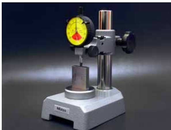
Reference point setting with a 50 mm Gauge Block.
