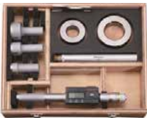
3-point internal micrometers with exchangeable measuring heads require new reference setting after an exchange of the measuring head.
