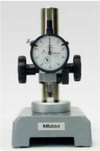
Zero setting with a 10 mm ceramic gauge block if the workpiece nominal is 10 mm
