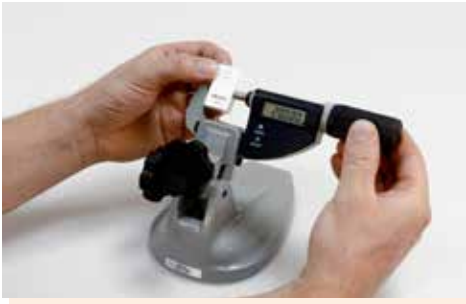
Reference point setting with a gauge block
