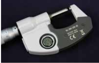
Rubber seal to protect the battery housing respectively output connector against ingress.
