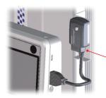
When attaching U-WAVE, the optional mounting plate (No. 02AZE990) is recommended.
